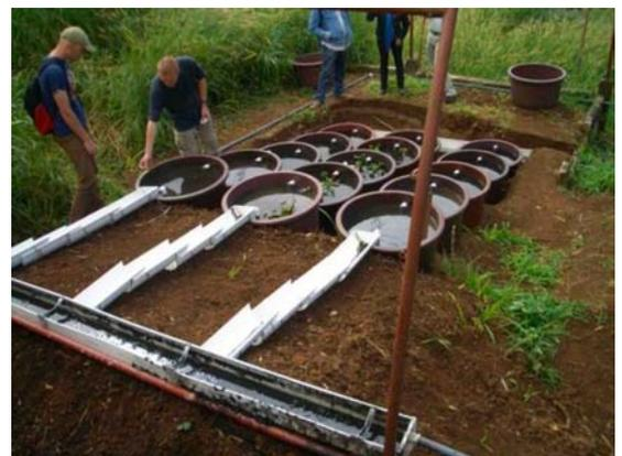
*Experimental system for treating effluent of anaerobic reactors*
