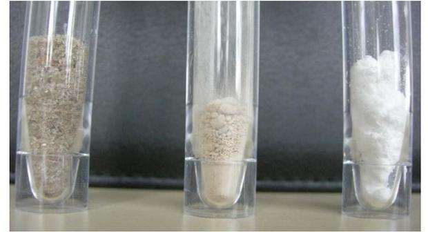
*Struvite precipitates from different processes*
