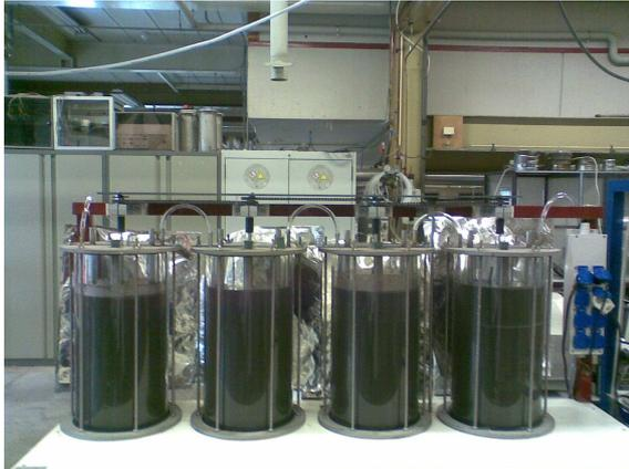
*Continuously Stirred Tank Reactors*
